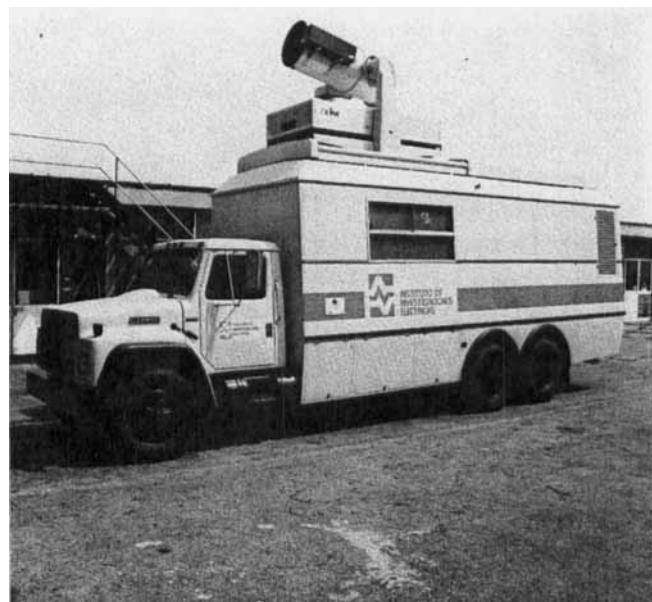
FIGURE 18. UV-visible DIAL system made by CISE for Instituto de Investigaciones Electricas, Mexico (IIE) for the detection of ozone and sulfur dioxide. The system parameters are reported in Table 1.
