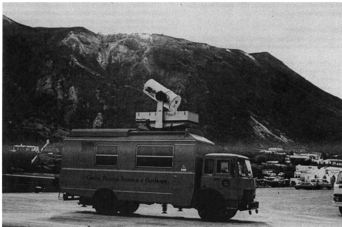
FIGURE 15. CISE-ENEL DIAL system. This picture was taken in 1983 during the campaign for the detection of sulfur dioxide emitted by the fumaroles of a volcano in Vulcano Island (Italy).
